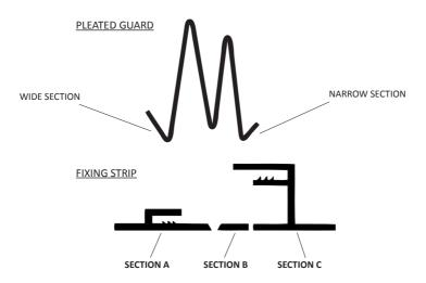
Use a stanley knife to cut the strip into sections A, B and C before commencing installation.
